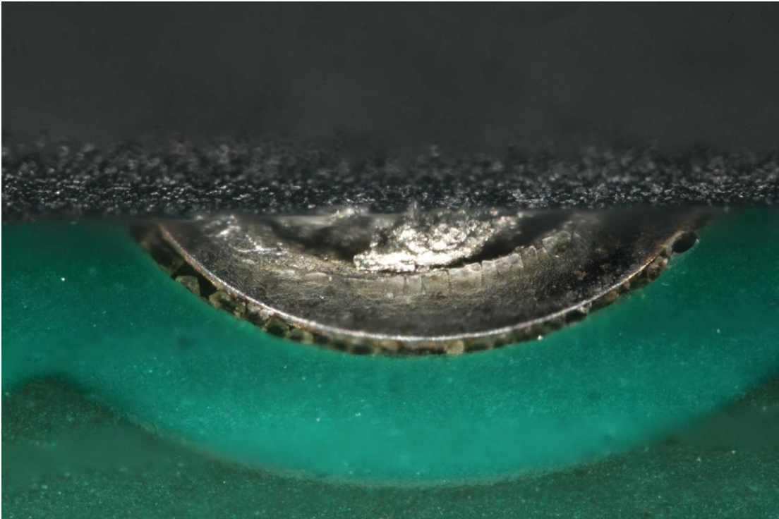
Figure 4. Specimen 4LP1 Visual inspection. Cracked solder visible beneath the component housing.
