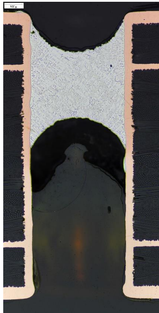
Figure 26. 103 Specimen 4LP1 Vias. No plating cracks, no voids, no nodules, no intrusions. Reasonably uniform plating thickness.
